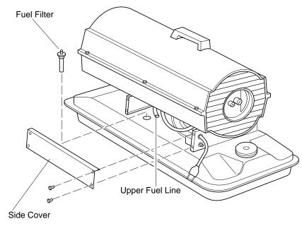
Figure 8 - Fuel Filter Removal
